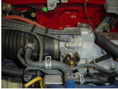
When I started, my intake manifold and throttle body looked like any other setup you might find on a 3rd generation Prelude. Obviously, the first thing you need to do is remove all the vacuum hoses from the throttle body and intake manifold.
