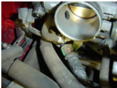
Next you'll need to remove the throttle body itself. This requires that you remove a few things that are holding it in place. A good place to start is to remove the wiring harness clip bolted to the bottom of the throttle -body. On my car, this clip had a green rubber jacket on it, making it easy to locate.
