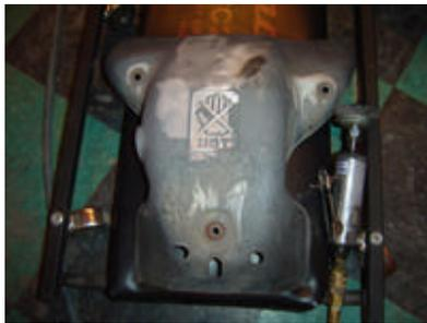
My solution to this problem was to unhook the power-steering line, allowing me a little more room. This worked well, and I was then able to remove it easily. Once I had it out, I sent it through the parts washer to clean all the dirt and oil off. This helped things a little bit, but the paint was still in terrible shape. Larger measures were needed!
